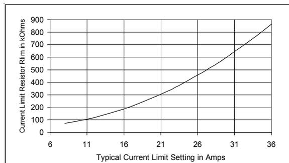
Fig. 6 Current Limit Adjustment using R<sub>LIM</sub>
