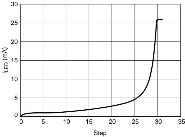
**Figure 4. Output Current Programmed Value ( I<sub>LED</sub> = F(Step) )**
