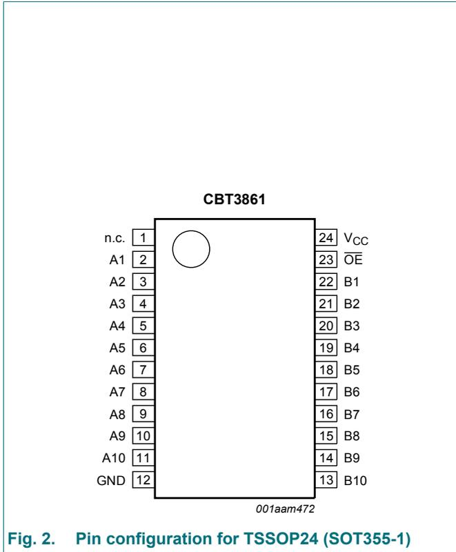
Fig. 2. Pin configuration for TSSOP24 (SOT355-1)
