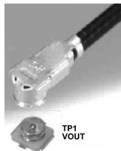
Figure 8. Technique for Measuring Output Ripple and Step Response with a Low Inductance Connector (Not Supplied)
