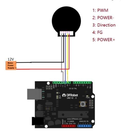
**NOTE**: Remember to connect Arduino GND to the POWER-.
