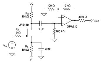
Figure 7-1. AC Measurement Reference Schematic
