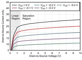
Figure 8-1. V<sub>DS</sub> vs I<sub>DS</sub>
