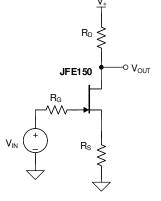
Figure 9-2. Common-Source Amplifier
