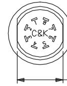
Terminal numbers molded on bottom of housing.
