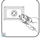
AC Input Connection: Insert L15-30P twist-lock plug into compatible L15-30R utility, generator or UPS outlet.
