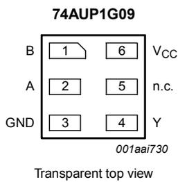
Figure 6. Pin configuration SOT891, SOT1115 and SOT1202
