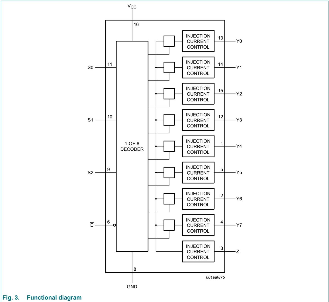
Fig. 3. Functional diagram
