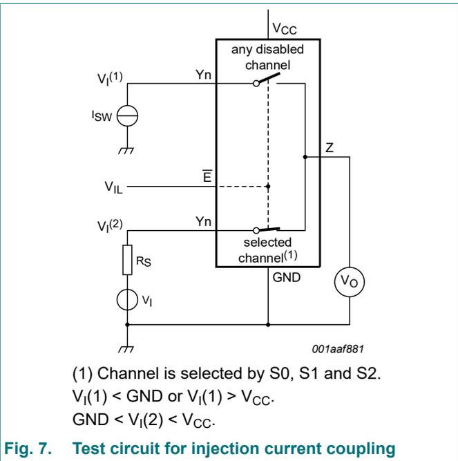
**Fig. 7. Test circuit for injection current coupling**
