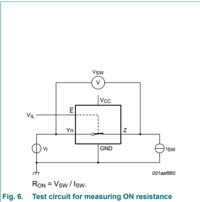
**Fig. 6. Test circuit for measuring ON resistance**
