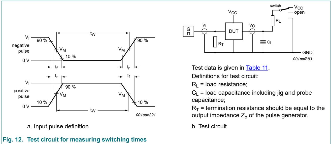
Fig. 12. Test circuit for measuring switching times
