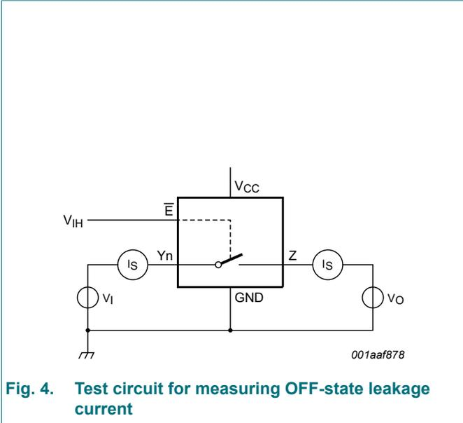
**Fig. 4. Test circuit for measuring OFF-state leakage current**
