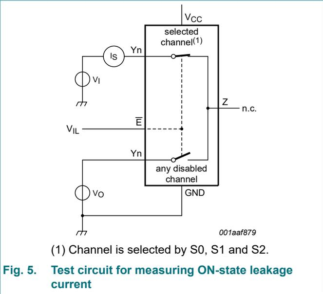
**Fig. 5. Test circuit for measuring ON-state leakage current**
