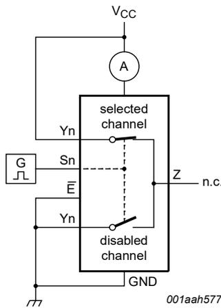
**Fig. 11. Test circuit for measuring power dissipation capacitance**
