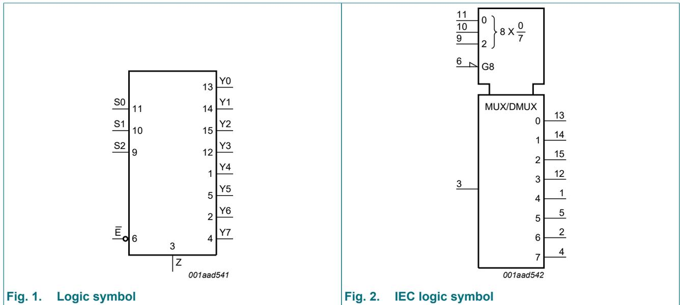
8-channel analog multiplexer/demultiplexer with injection-current effect control
