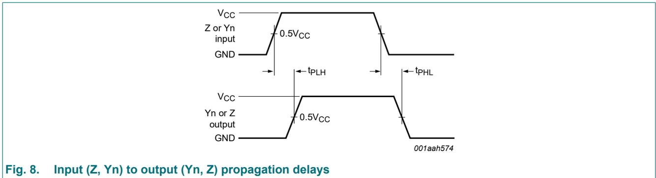
Fig. 8. Input (Z, Y<sub>n</sub>) to output (Y<sub>n</sub>, Z) propagation delays
