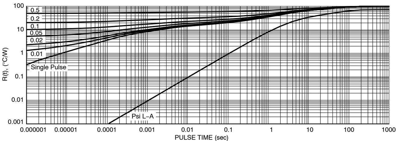
Figure 29. Transient Thermal Response (SOIC-8 Fused)
