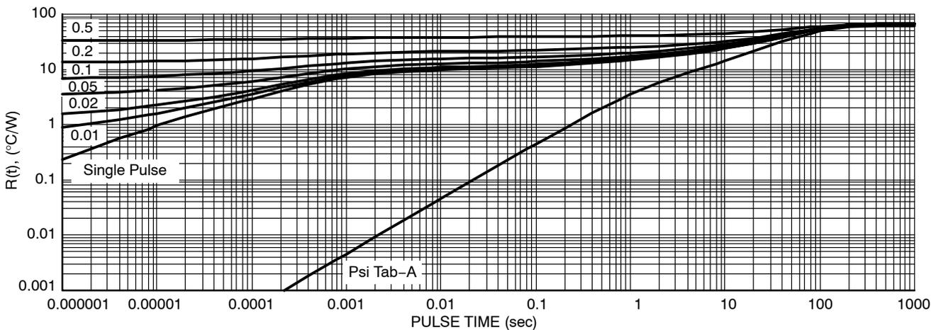
Figure 27. Transient Thermal Response (DPAK)
