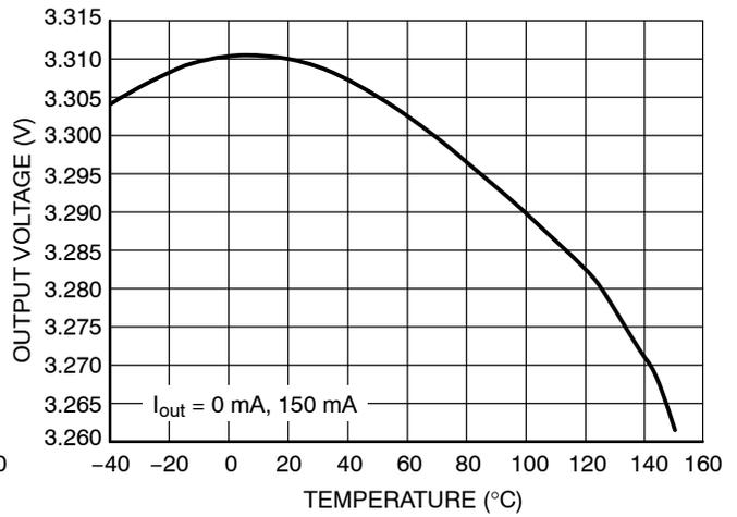
Figure 4. Output Voltage vs. Temperature (OUT = 3.3 V)
