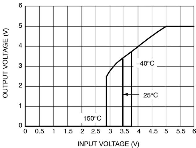
Figure 7. Output Voltage vs. Input Voltage (R<sub>LOAD</sub> = 51 k, I<sub>out</sub> = 100 μA, OUT = 5 V)
