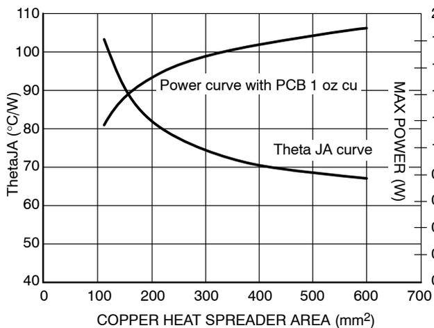
Figure 26.  $R_{\theta JA}$  vs. PCB Copper Area (DPAK)
