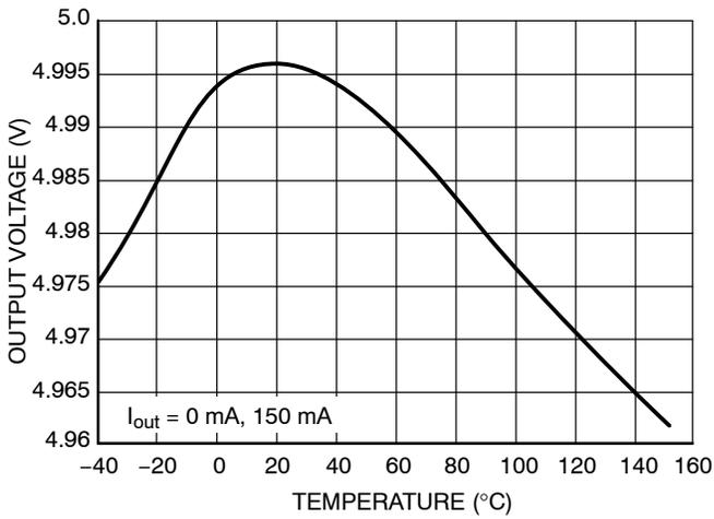
Figure 3. Output Voltage vs. Temperature (OUT = 5 V)
