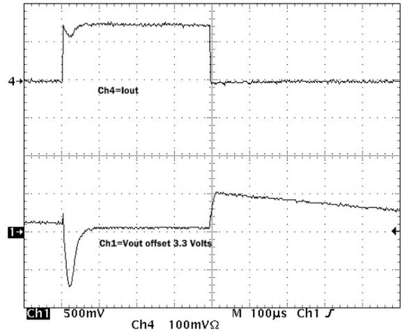
Figure 17. Load Transient
