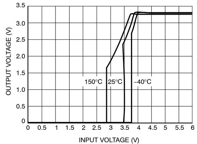
Figure 8. Output Voltage vs. Input Voltage (R<sub>LOAD</sub> = 51 k, I<sub>out</sub> = 100 μA, OUT = 3.3 V)
