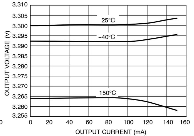
Figure 6. Output Voltage vs. Output Current (OUT = 3.3 V)
