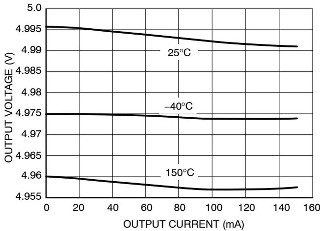
Figure 5. Output Voltage vs. Output Current (OUT = 5 V)
