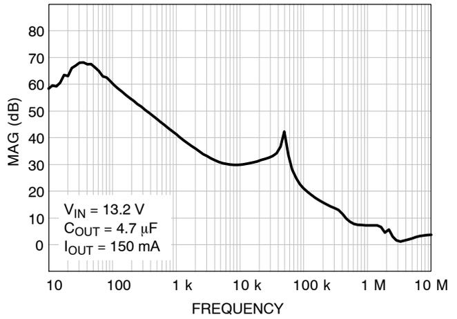
Figure 20. Ripple Rejection vs. Frequency
