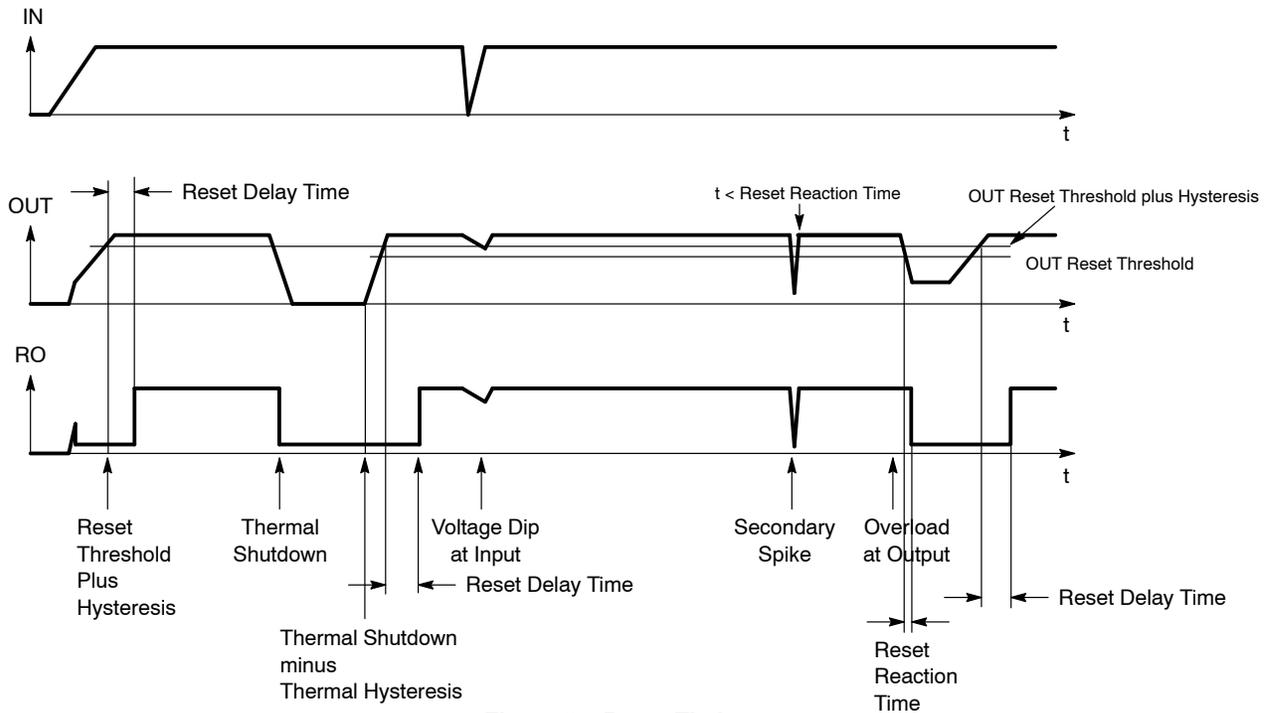
**Figure 25. Reset Timing**
