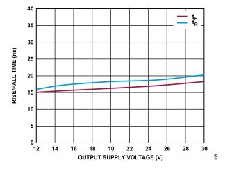
Figure 12. Rise and Fall Time vs. Output Supply Voltage ( $V_{DD2}$ ),  $V_{DD1}$  = 5 V, 2 nF Load,  $R_G$  = 3.6  $\Omega$
