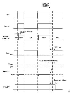
Figure 17. Desaturation Detection Timing Diagram
