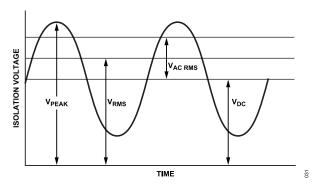
Figure 21. Critical Voltage Example
