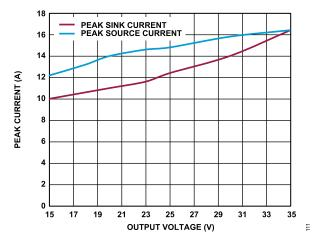
Figure 15. Peak Current vs. Output Voltage, 0 Ω Series Gate Resistor
