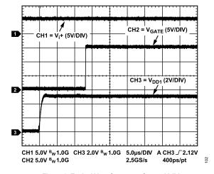
Figure 6. Typical V<sub>DD1</sub> Startup to Output Valid
