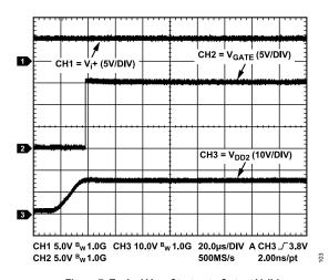
Figure 7. Typical V<sub>DD2</sub> Startup to Output Valid
