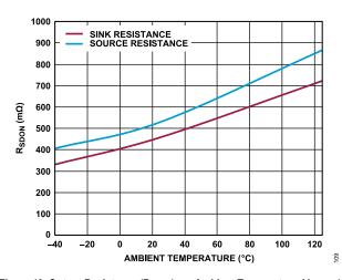
Figure 13. Output Resistance ( $R_{DSON}$ ) vs. Ambient Temperature,  $V_{DD2}$  = 15 V, 250 mA Test
