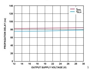
Figure 11. Propagation Delay vs. Output Supply Voltage ( $V_{DD2}$ ),  $V_{DD1} = 5 \text{ V}$
