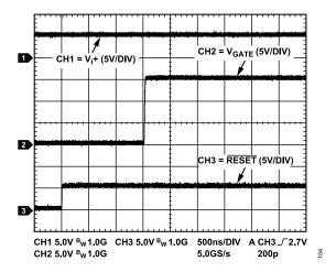
Figure 8. Typical RESET to Output Valid
