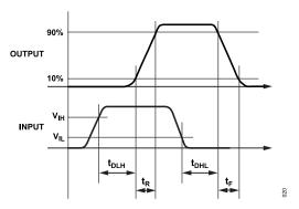
Figure 16. Propagation Delay Parameters
