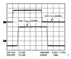
Figure 4. Typical Input to Output Waveform, 2 nF Load, 3.6  $\Omega$  Series Gate Resistor,  $V_{DD1}$  = 5 V,  $V_{DD2}$  = 15 V,  $V_{SS2}$  = -5 V
