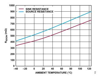
Figure 14.  $R_{DSON}$  vs. Ambient Temperature,  $V_{DD2}$  = 15 V, 1 A Test
