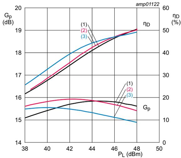
$V_{DS} = 30\text{ V}; I_{Dq} = 300\text{ mA}; V_{GS(amp)peak} = 1.1\text{ V}.$
