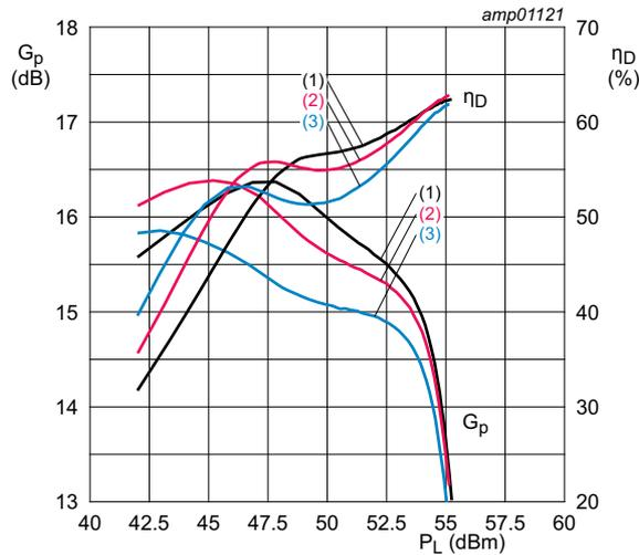
$V_{DS} = 30\text{ V}$ ;  $I_{Dq} = 300\text{ mA}$ ;  $V_{GS(amp)peak} = 1.1\text{ V}$ ;  $t_p = 100\text{ }\mu\text{s}$ ;  $\delta = 10\text{ }\%$ .
