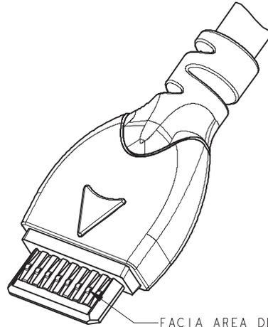
FACIA AREA DESIGNED TO ALLOW FOR SOCKET CONNECTOR TO BE RECESSED IN CASING
