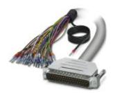
Assembled shielded round cable; connection 1: Single wires (37-position) (The wires are marked and fitted with ferrules. The braided shield is routed to a separate cable end.); connection 2: D-SUB pin strip (1x 37-position); cable length: 1 m
