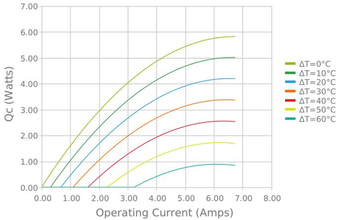
Heat Pumped at Cold Side
