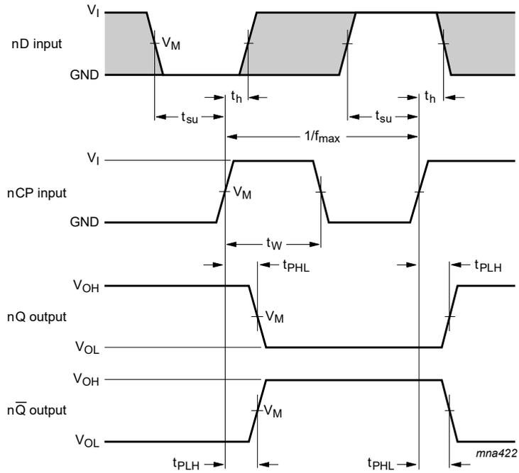
The shaded areas indicate when the input is permitted to change for predictable output performance.
