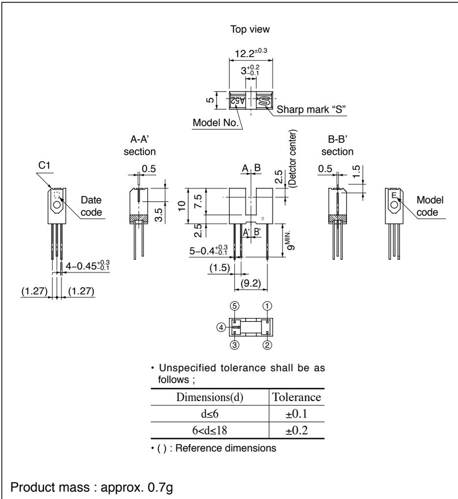
Dip soldering material : Sn-3Ag-0.5Cu
