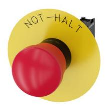
EMERGENCY STOP mushroom-type actuator, 22 mm, round, plastic, red, 40 mm, positive latching, according to EN ISO 13850, pull-to-unlatch mechanism, with yellow backing plate, inscription: NOT-HALT, with holder, 1 NC, screw terminal, Z=20-unit packaging
