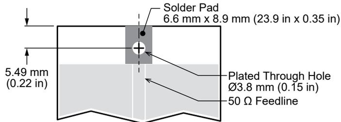
Figure 2. ANT-8/9-PW-LPN Recommended Mounting and PCB Footprint
