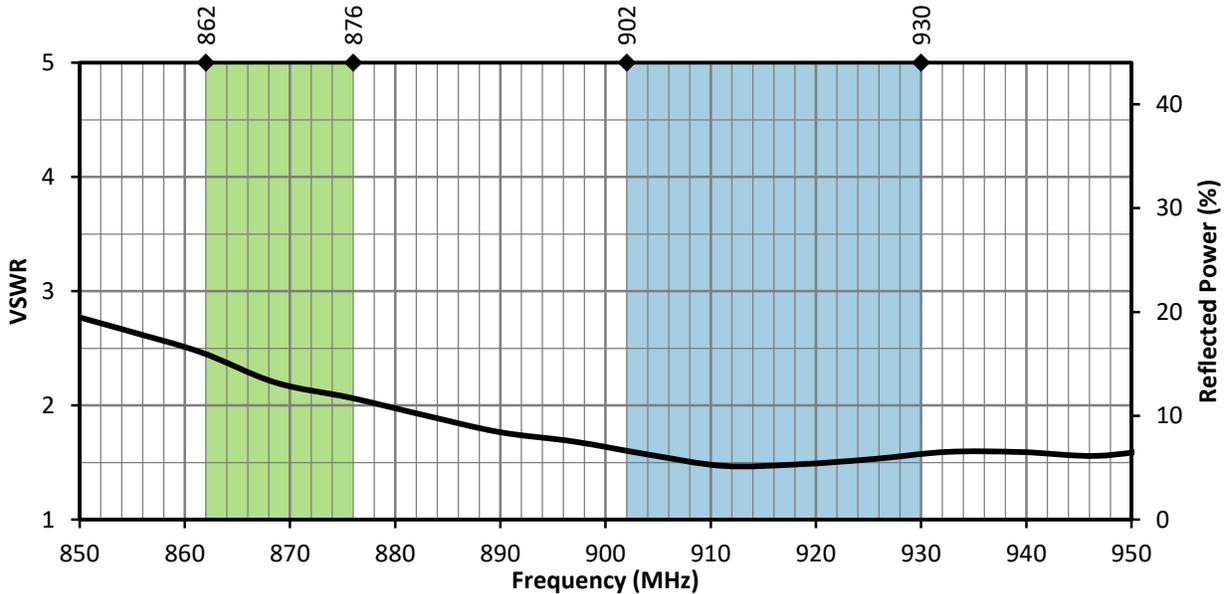
Figure 4. VSWR for ANT-8/9-PW-LPN, Edge of ground Plane
