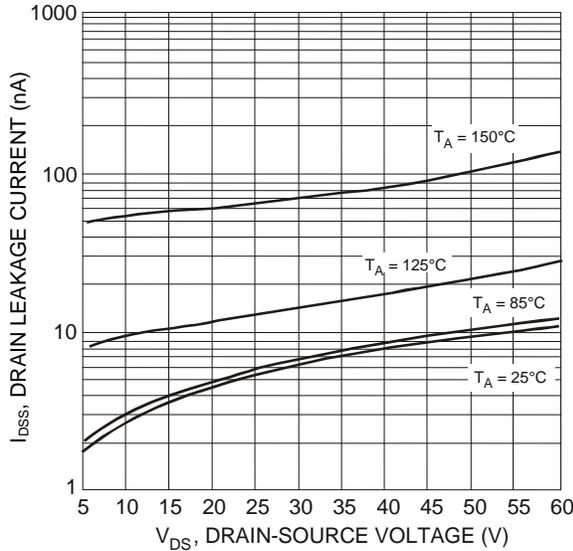
Figure 7 Typical Drain-Source Leakage Current vs. Voltage
