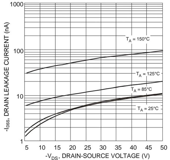
Figure 14 Typical Drain-Source Leakage Current vs. Voltage
