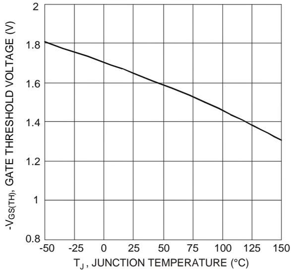
Figure 15 Gate Threshold Variation vs. Junction Temperature
