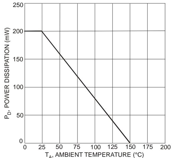
Figure 6 Max Power Dissipation vs. Ambient Temperature
