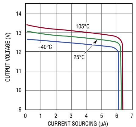
**V<sub>OUT\_EN[0:3]</sub> and AUXFAULTB VOL vs Load Current**
