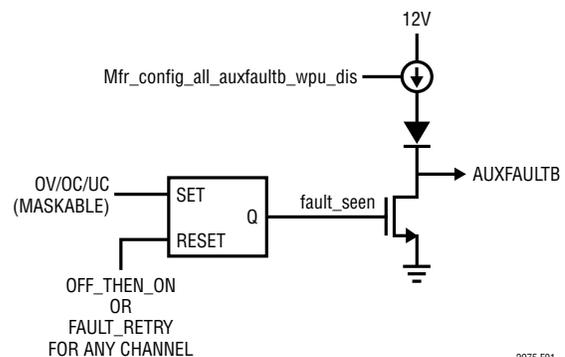
Figure 1. AUXFAULTB MUX
