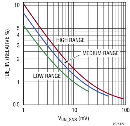
Figure 27. TUE\_IIN vs READ\_IIN Input Voltage in Percentage
