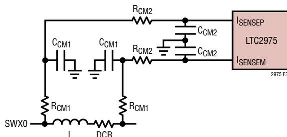
Figure 38. DCR Current Sensing Circuits
