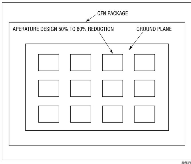
Figure 46. Suggested Screen Pattern for Die Attach Pad
