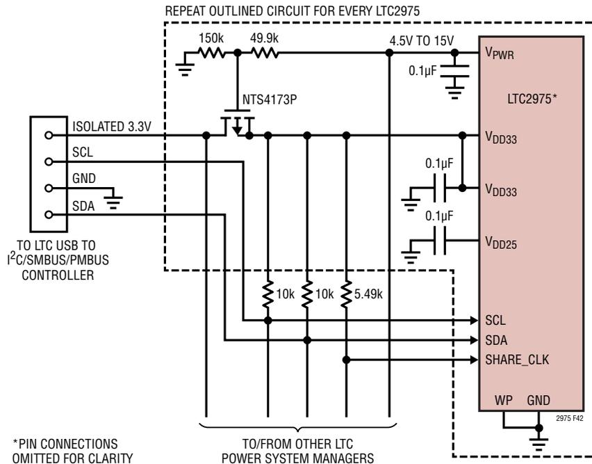
Figure 42. ADI Controller Connections When V<sub>PWR</sub> Is Used
