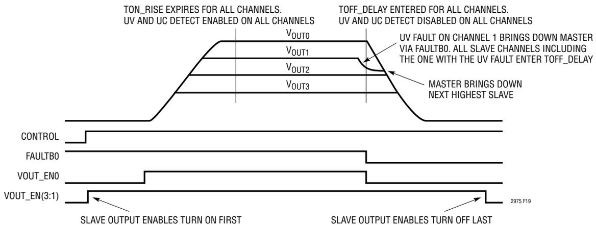
**Figure 19. Fault on Channel 1 Tracking All Supplies Down**
