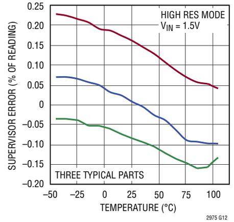
**Current Supervisor Total Unadjusted Error vs Temperature**
