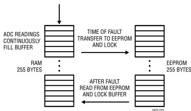
Figure 22. Fault Logging
