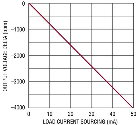
**V<sub>OUT\_EN[0:3]</sub> and AUXFAULTB Output High Voltage vs Load Current**
