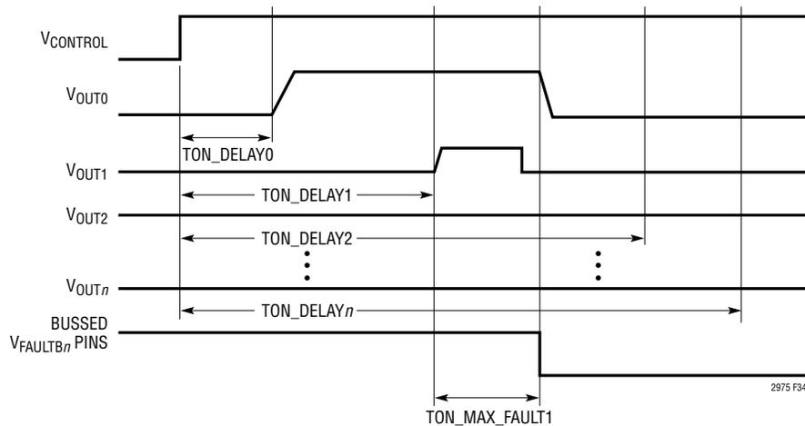
Figure 34. Aborted On-Sequence Due to Channel 1 Short
