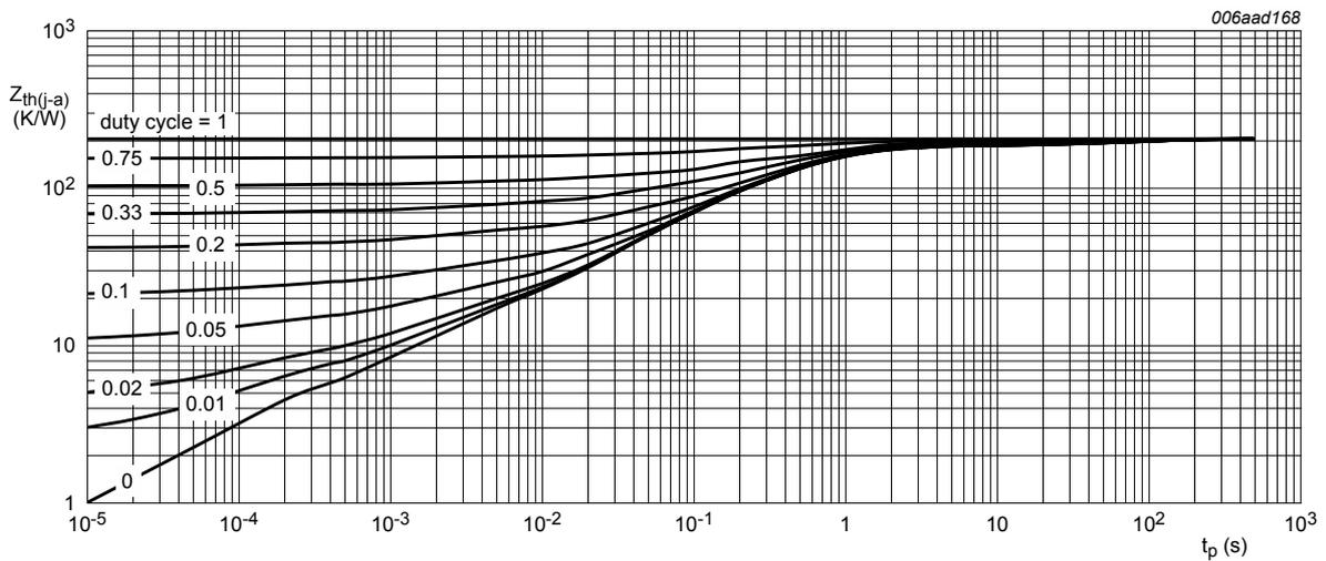
4-layer PCB 35  $\mu\text{m}$ , standard footprint
