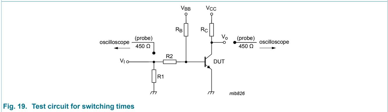
Fig. 19. Test circuit for switching times
