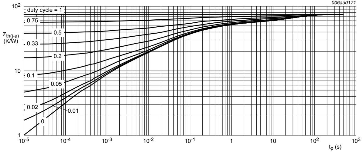
4-layer PCB 70  $\mu\text{m}$ , mounting pad for collector 1  $\text{cm}^2$
