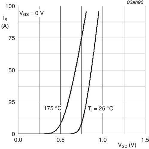
$T_j = 25^\circ\text{C}$  and  $175^\circ\text{C}; V_{GS} = 0\text{V}$
