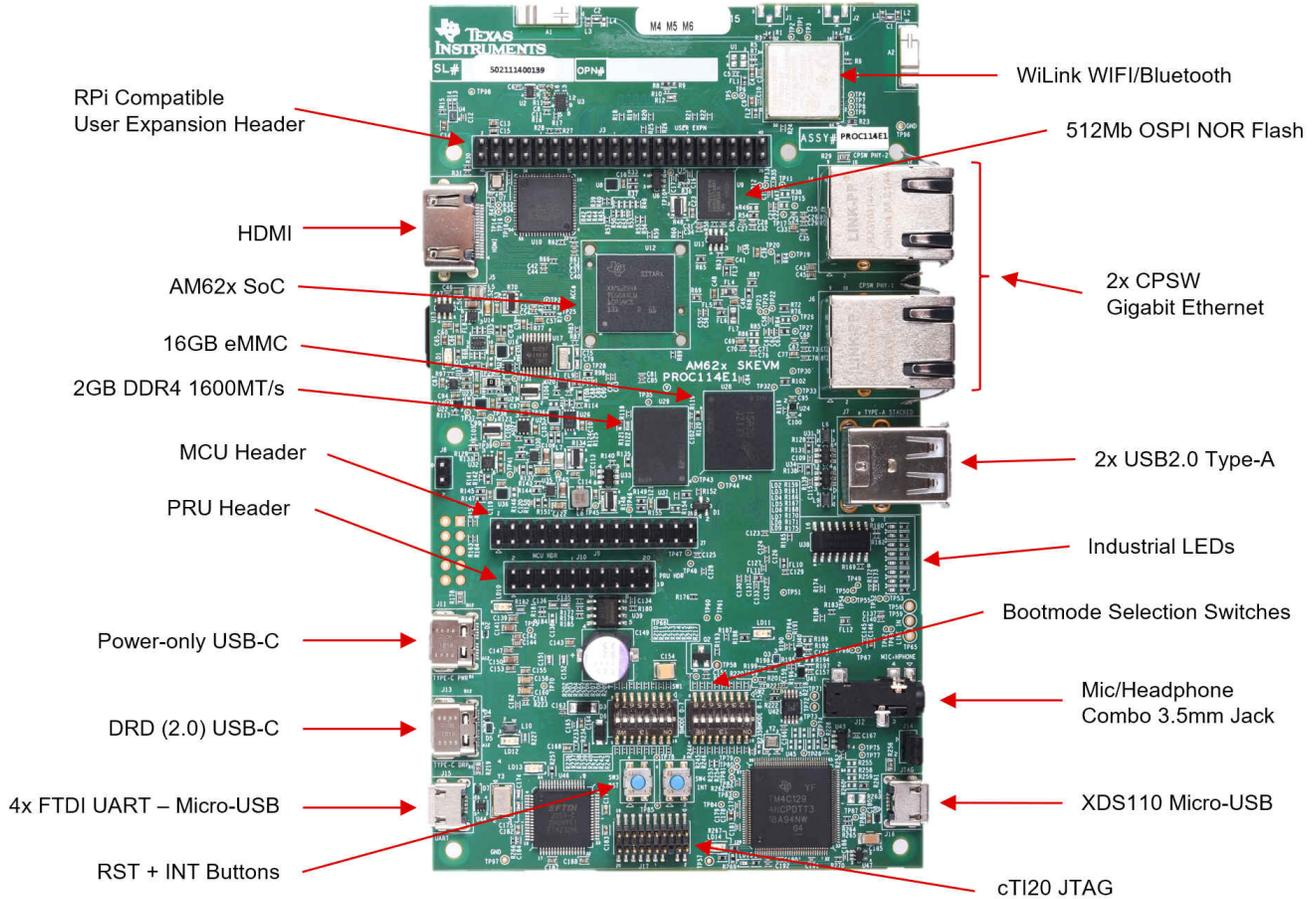
Figure 2-1. SK-AM62 Top View
