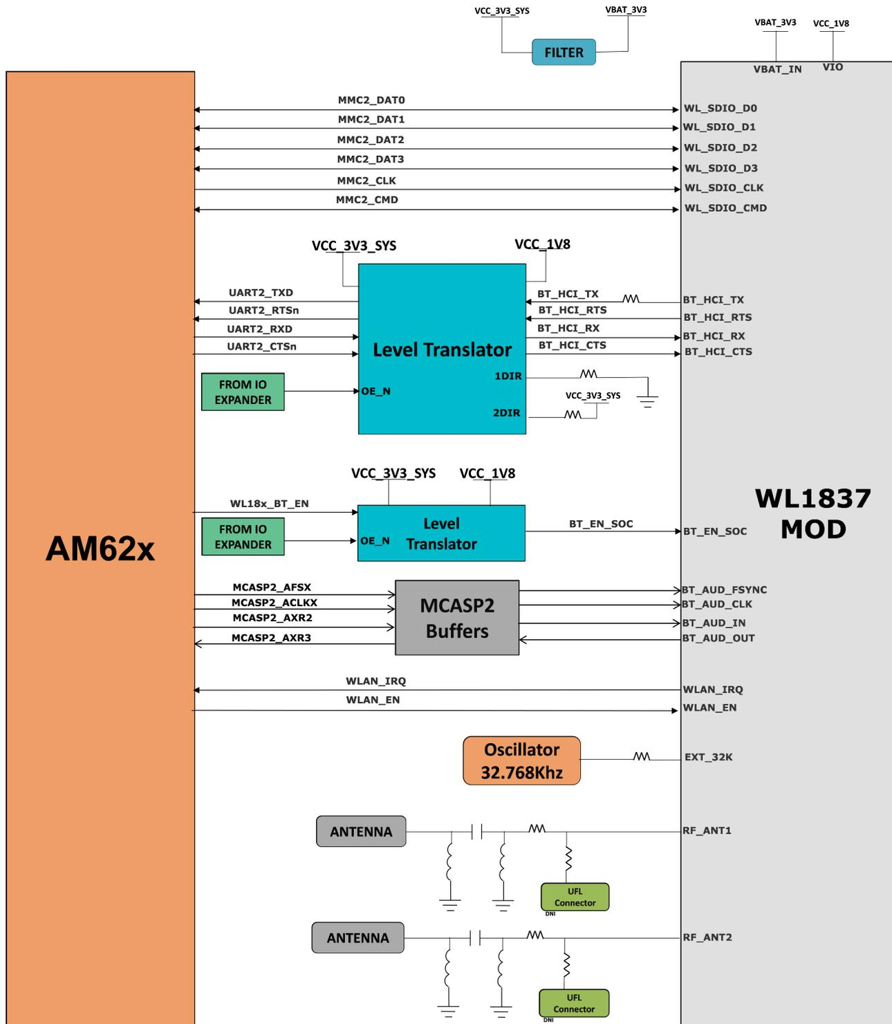
Figure 2-11. MMC2 - Wilink Interface on SK-AM62 and SK-AM62-P1
