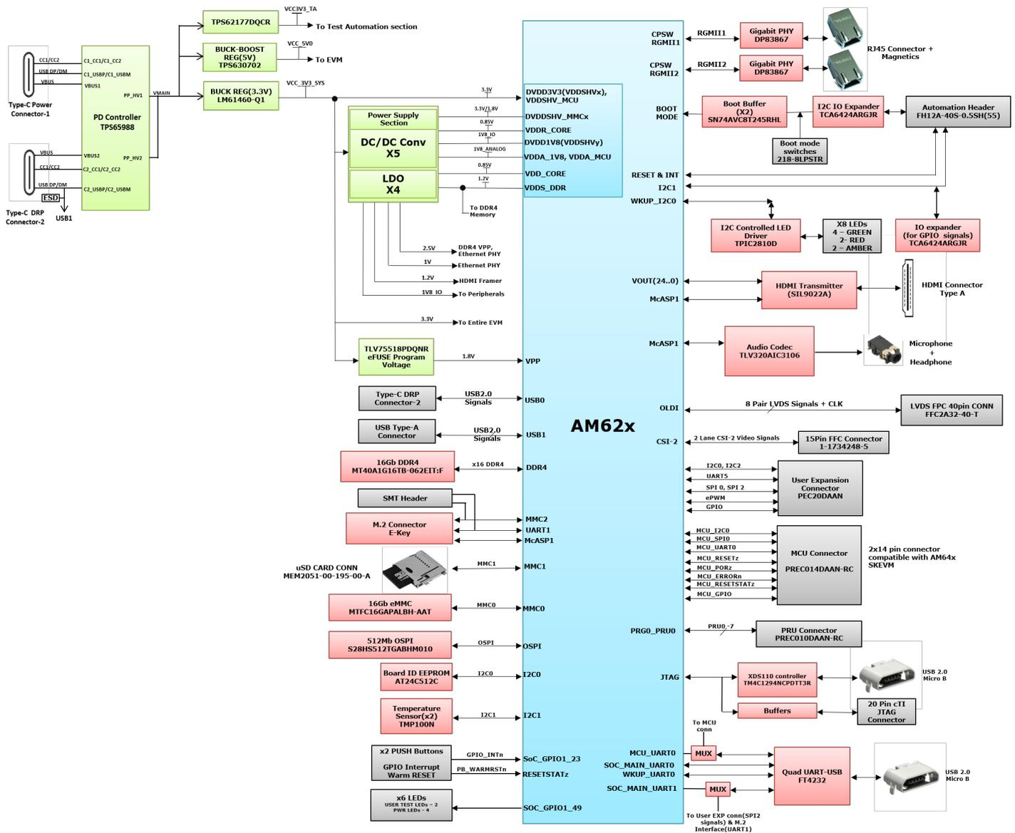
Figure 2-4. Functional Block Diagram of the SK-AM62B Board
