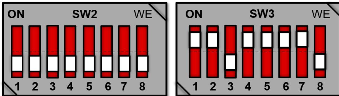
Figure 2-7. SD Bootmode Switch Setting Example (From E2)
