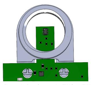
Figure 5-23. Base Connected to TMAG5328EVM
