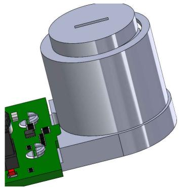
Figure 5-25. Screw Fully Fastened Into Base
