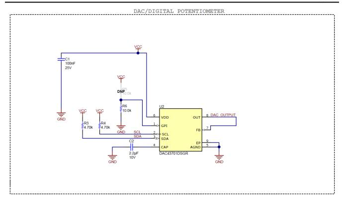
Figure 4-2. Schematic Snippet of DAC43701 Portion of TMAG5328EVM
