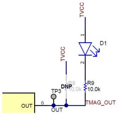
Figure 5-21. OUT LED Circuit
