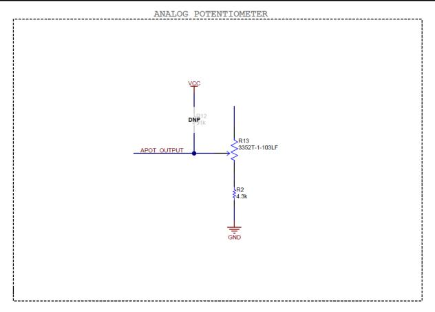
Figure 4-3. Schematic Snippet of Potentiometer Portion of TMAG5328EVM
