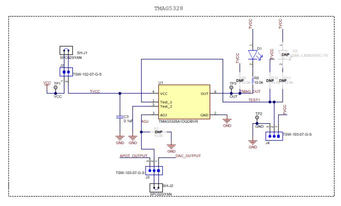
Figure 4-1. Schematic Snippet of TMAG5328 Portion of TMAG5328EVM
