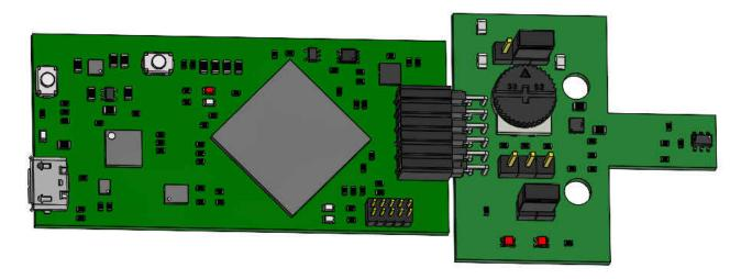
Figure 5-1. Sensor Control Board Connected to TMAG5328EVM
