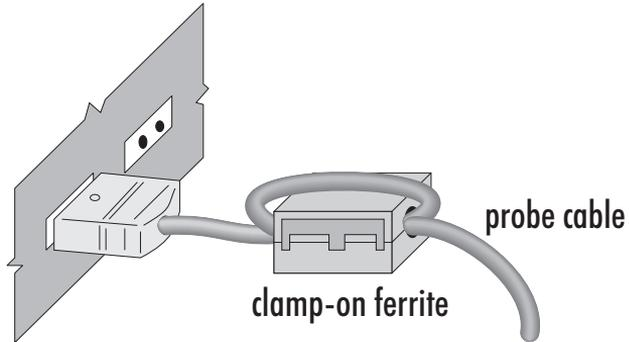
*Figure 1* Clamp-On Ferrite
