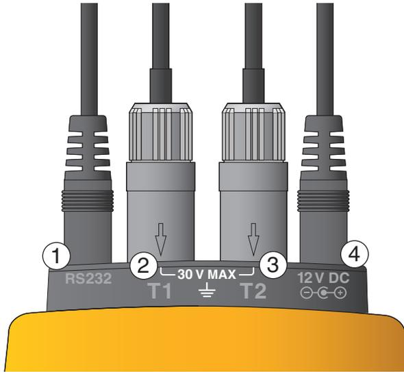
Figure 3 Input/Output Connections - 1524
