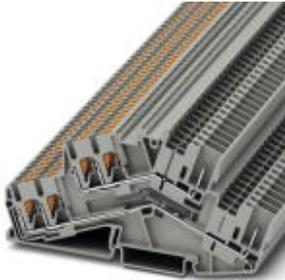
Double-level terminal block, Cross section: 0.14 mm<sup>2</sup> - 4 mm<sup>2</sup>, AWG: 26 - 12, Connection type: Push-in connection, Width: 5.2 mm, Color: blue, Mounting type: NS 35/7,5, NS 35/15
