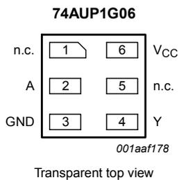
Figure 6. Pin configuration SOT891, SOT1115 and SOT1202 (XSON6)
