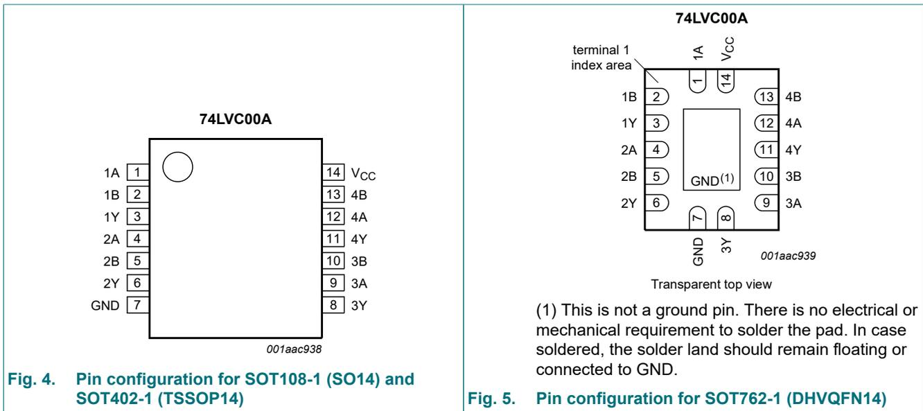
Fig. 4. Pin configuration for SOT108-1 (SO14) and SOT402-1 (TSSOP14)
