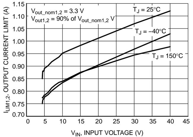
Figure 9. Output Current Limit vs. Input Voltage
