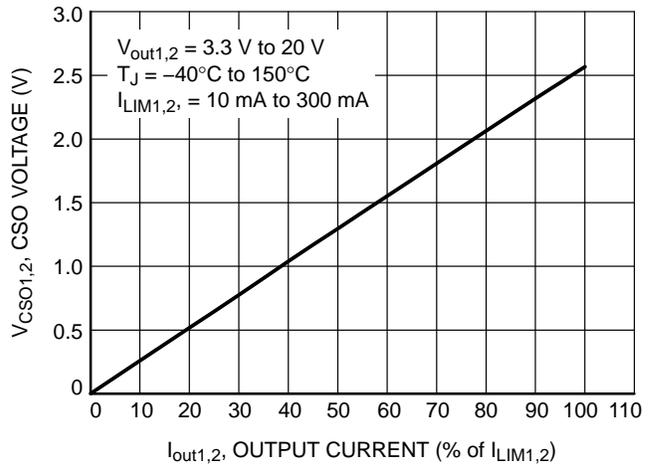
Figure 11. Output Current (% of  $I_{LIM}$ ) vs. CSO Voltage
