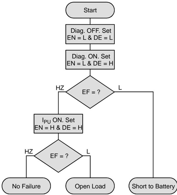
Figure 20. Flowchart for Diagnostics in OFF State
