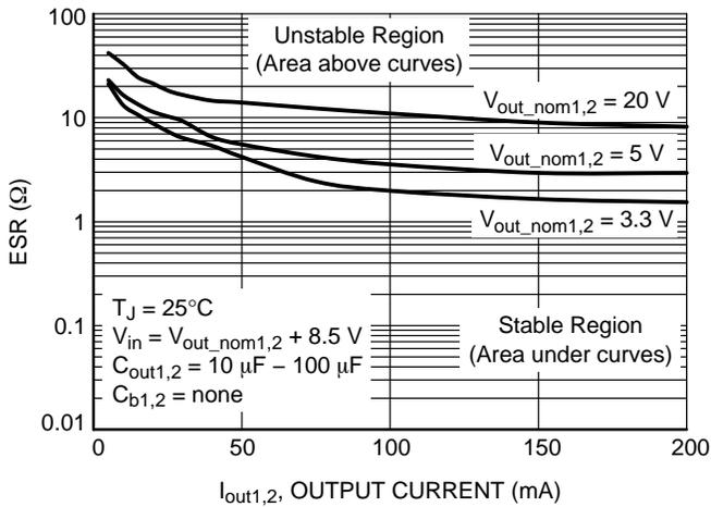
Figure 16. Output Capacitor Stability Region vs. Output Current
