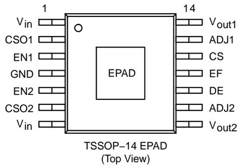
**Figure 3. Pin Connections**
