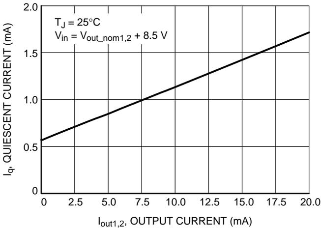
Figure 12. Quiescent Current vs. Output Current (Low Load)
