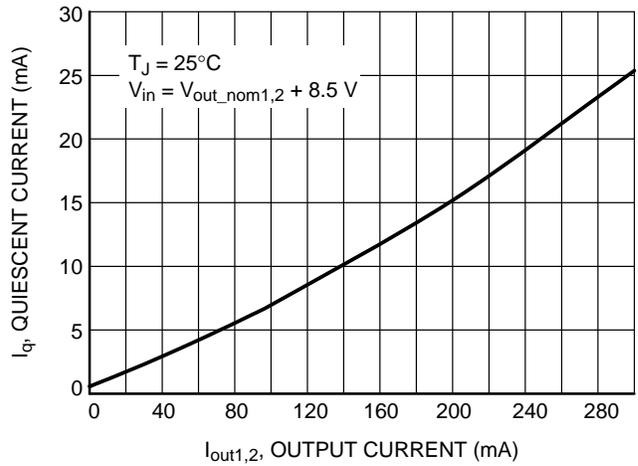
Figure 13. Quiescent Current vs. Output Current (High Load)
