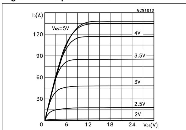
Figure 5. Transfer characteristics
