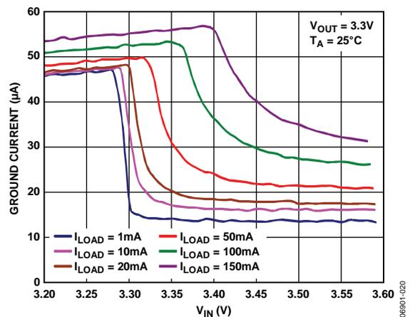
Figure 16. Ground Current vs. Input Voltage (In Dropout)
