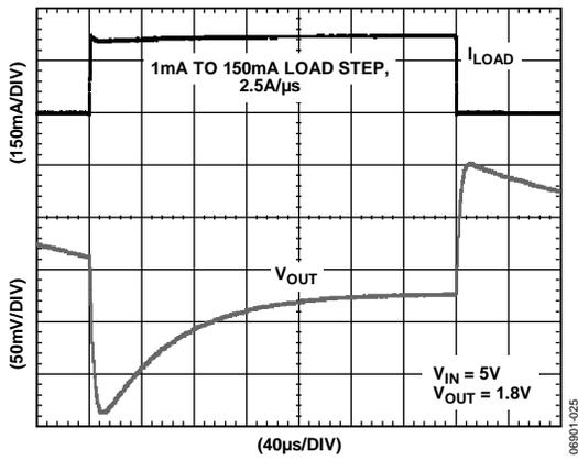
Figure 24. Load Transient Response,  $C_{IN} = C_{OUT} = 4.7 \mu F$
