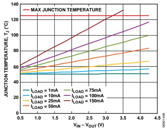
Figure 44. WLCSP, 100 mm<sup>2</sup> of PCB Copper, T<sub>A</sub> = 50°C
