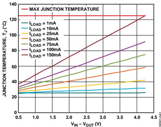
Figure 41. WLCSP, 100 mm<sup>2</sup> of PCB Copper, T<sub>A</sub> = 25°C
