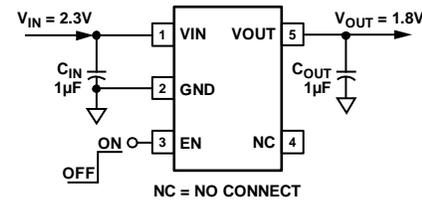
Figure 1. ADP121 TSOT with Fixed Output Voltage, 1.8 V
