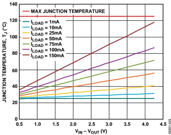
Figure 35. TSOT, 100 mm<sup>2</sup> of PCB Copper, T<sub>A</sub> = 25°C
