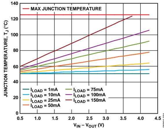
Figure 37. TSOT, 500 mm<sup>2</sup> of PCB Copper, T<sub>A</sub> = 50°C
