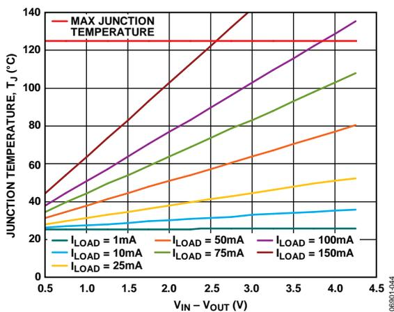
Figure 42. WLCSP, 0 mm<sup>2</sup> of PCB Copper, T<sub>A</sub> = 25°C
