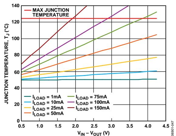
Figure 45. WLCSP, 0 mm<sup>2</sup> of PCB Copper, T<sub>A</sub> = 50°C
