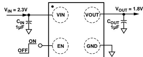
Figure 2. ADP121 WLCSP with Fixed Output Voltage, 1.8 V
