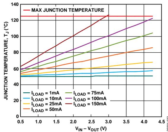
Figure 39. TSOT, 0 mm<sup>2</sup> of PCB Copper, T<sub>A</sub> = 50°C
