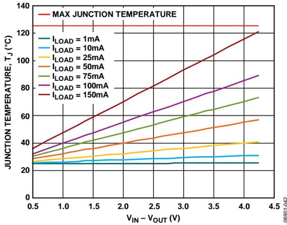
Figure 40. WLCSP, 500 mm<sup>2</sup> of PCB Copper, T<sub>A</sub> = 25°C
