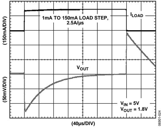
Figure 23. Load Transient Response,  $C_{IN} = C_{OUT} = 1 \mu F$
