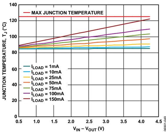
Figure 47. WLCSP, 100 mm<sup>2</sup> of PCB Copper, Board Temperature = 85°C
