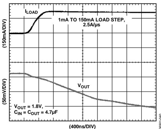
Figure 29. Output Transient Response,  $C_{OUT} = 4.7 \mu\text{F}$
