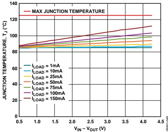
Figure 46. TSOT, 100 mm<sup>2</sup> of PCB Copper, Board Temperature = 85°C
