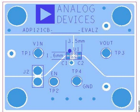
Figure 49. Example of WLCSP PCB Layout—Top Side
