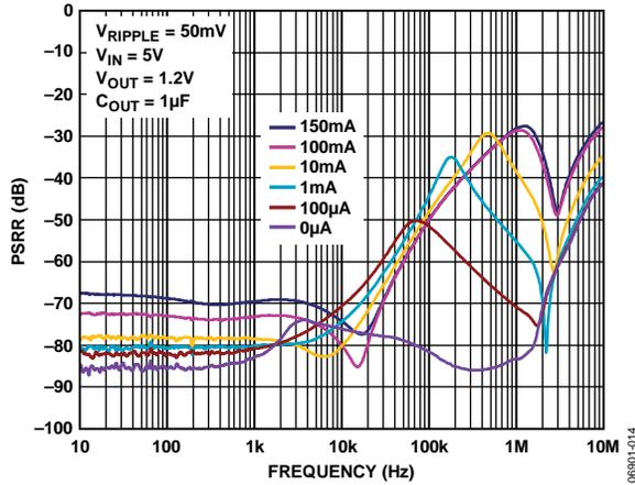
Figure 17. Power Supply Rejection Ratio vs. Frequency
