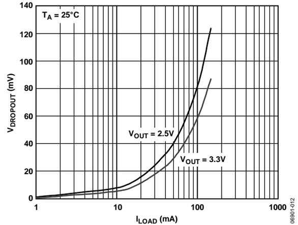
Figure 14. Dropout Voltage vs. Load Current, WLCSF
