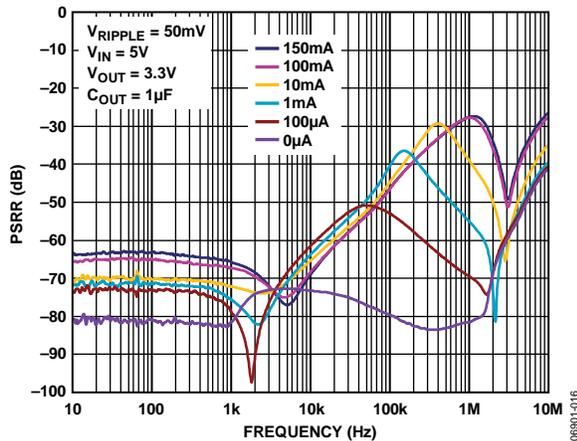
Figure 19. Power Supply Rejection Ratio vs. Frequency
