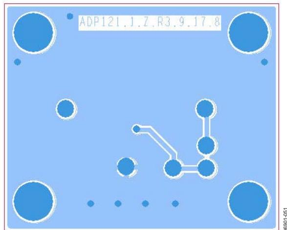
Figure 50. Example of WLCSP PCB Layout—Bottom Side
