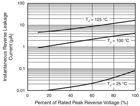
Fig. 4 - Typical Reverse Leakage Characteristics Per Diode
