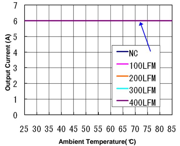
**Figure 8(d).** Current Derating Curve for 2.5V Output
