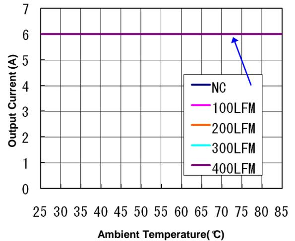
**Figure 8(b).** Current Derating Curve for 1.2V Output
