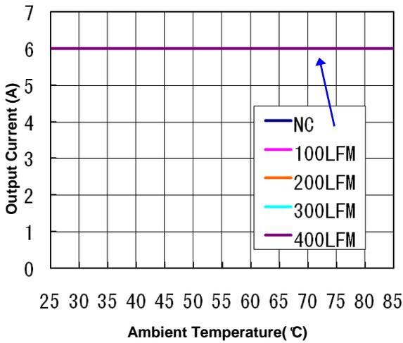
**Figure 8(a).** Current Derating Curve for 0.59V
