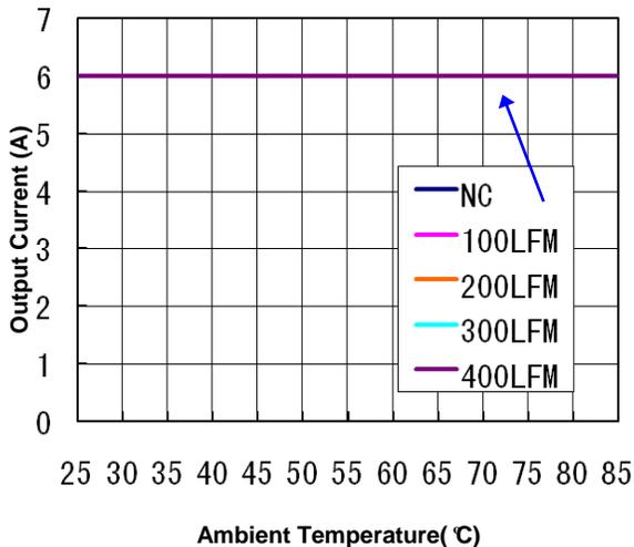
**Figure 8(e).** Current Derating Curve for 3.3V Output
