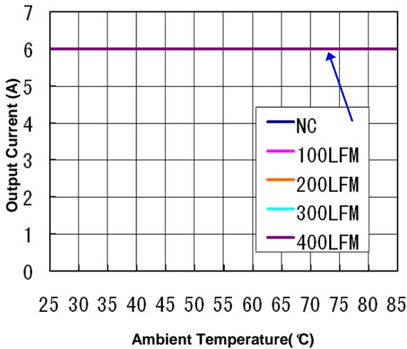
**Figure 8(c).** Current Derating Curve for 1.8V Output
