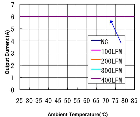
**Figure 8(f).** Current Derating Curve for 5V Output
