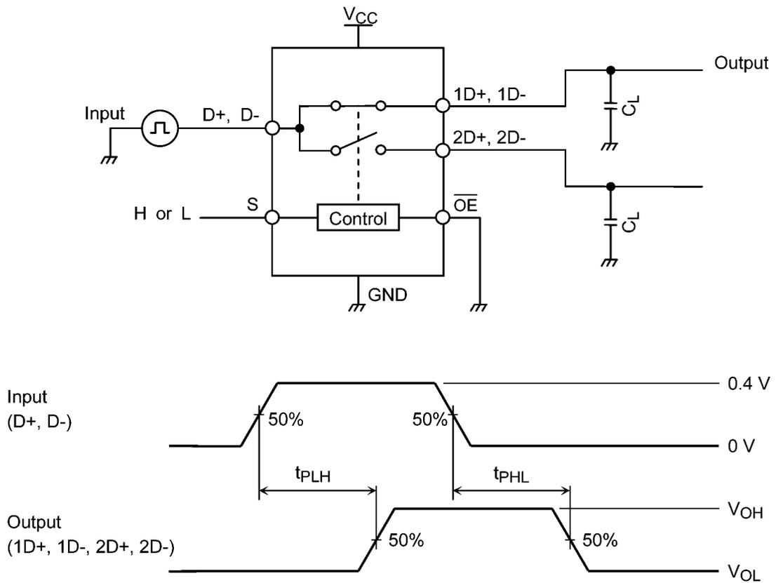
Fig. 11.1 Propagation Delay Time (t<sub>PLH</sub>, t<sub>PHL</sub>)
