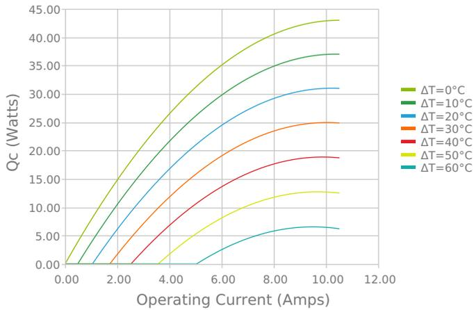
Heat Pumped at Cold Side
