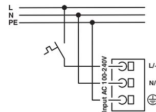
Figure 12 Schematic diagram, switching the input terminals
