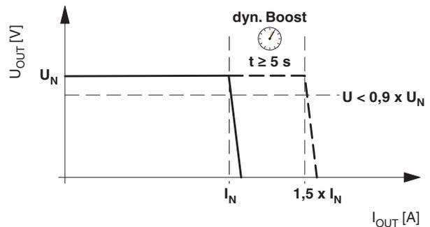
Figure 15  $U/I$  characteristic curve with dynamic load reserve
