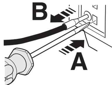
Figure 9 Release connecting cable (push-in connection technology)
