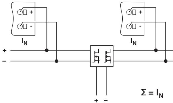
Figure 23 Schematic diagram, decoupling with ORING module
