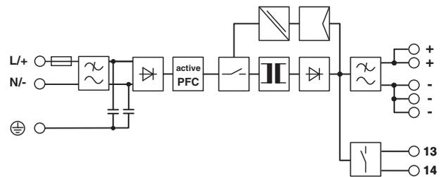
Figure 1 Block diagram
