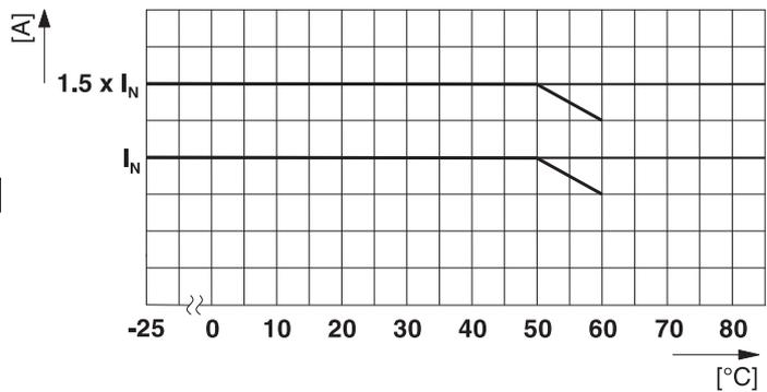
Rotated mounting position 180° X-axis
