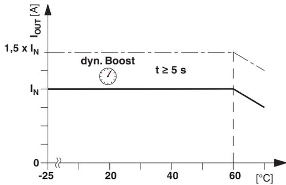
Figure 19 Temperature derating in normal mounting position
