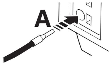
Figure 8 Insert connecting cable (push-in connection technology)
