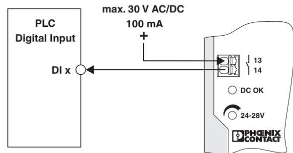
Figure 18 Wiring principle
