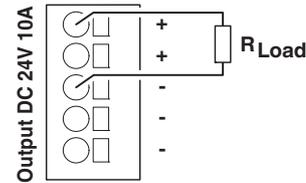
Figure 14 Schematic diagram, switching the output terminals
