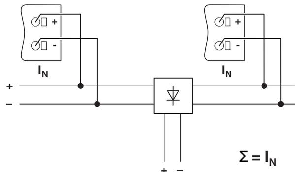
Figure 22 Schematic diagram, decoupling with diode module
