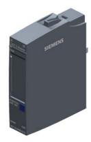
SIMATIC ET 200SP, Analog input module, Al 2x U/I 2-.4-wire High Feat., suitable for BU type A0, A1, Color code CC05, channel diagnostics, 16 bit, +/-0.1%
