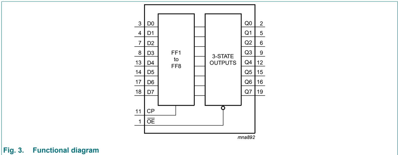
Octal D-type flip-flop; 5 V tolerant inputs/outputs; positive-edge trigger; 3-state
