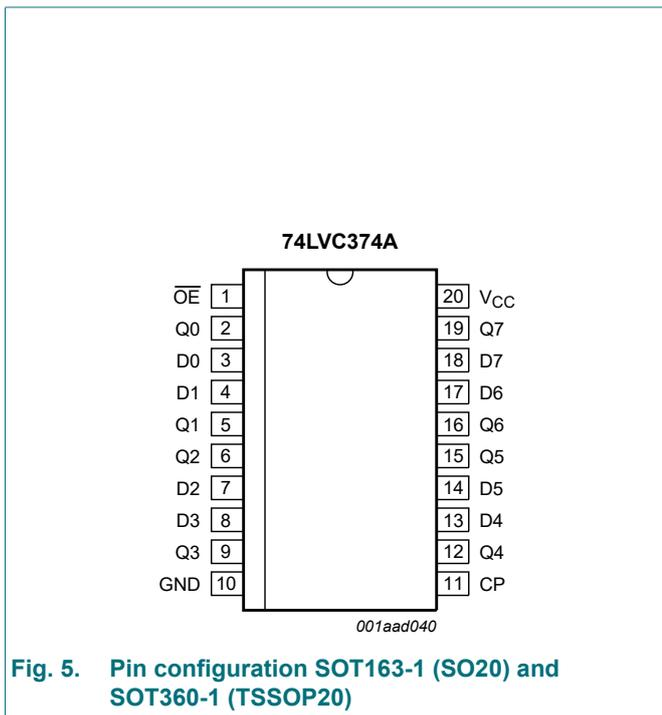
Fig. 5. Pin configuration SOT163-1 (SO20) and SOT360-1 (TSSOP20)
