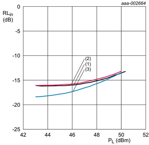
$V_{DS} = 28\text{ V}; I_{Dq} = 1200\text{ mA}.$
