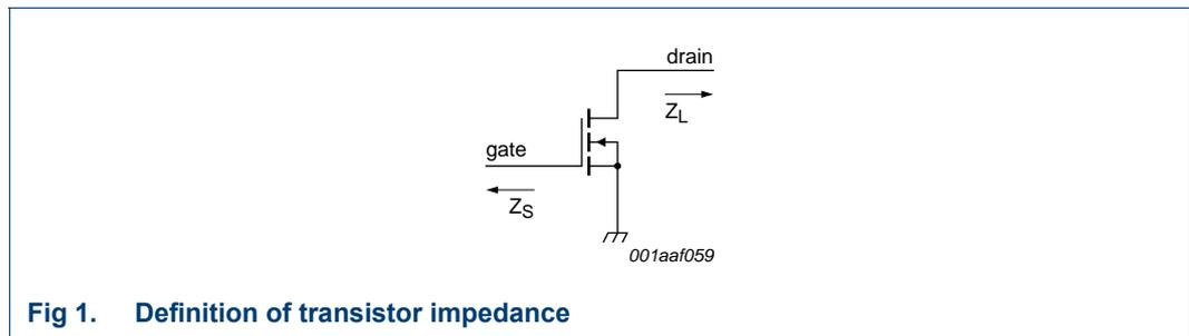
Fig 1. Definition of transistor impedance
