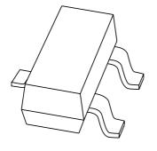
PBSS8110T 100 V, 1 A NPN low V<sub>CEsat</sub> (BISS) transistor
