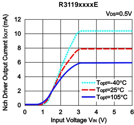
13) Nch Driver Output Current vs.  $V_{DS}$
