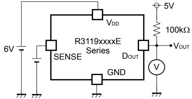
**Detector Threshold Test Circuit**
