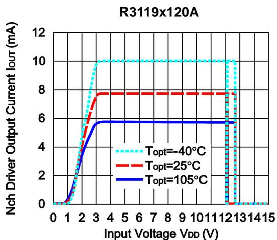
5) Nch Driver Output Current vs.  $V_{DS}$
