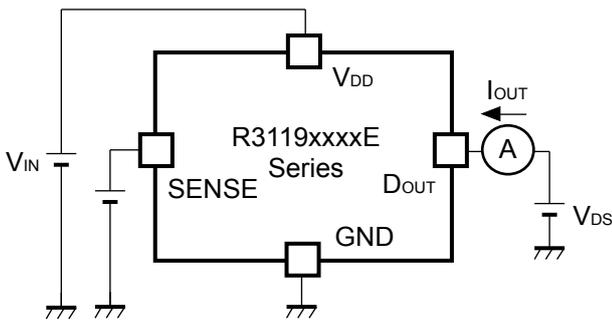
**Nch Driver Output Current Test Circuit**
