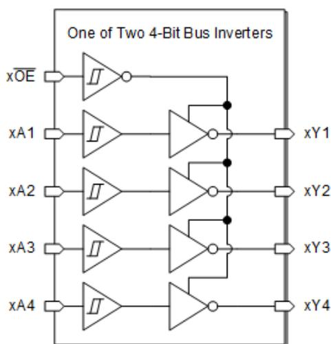
Figure 8-1. Logic Diagram (Positive Logic) for SN74HCS240-Q1
