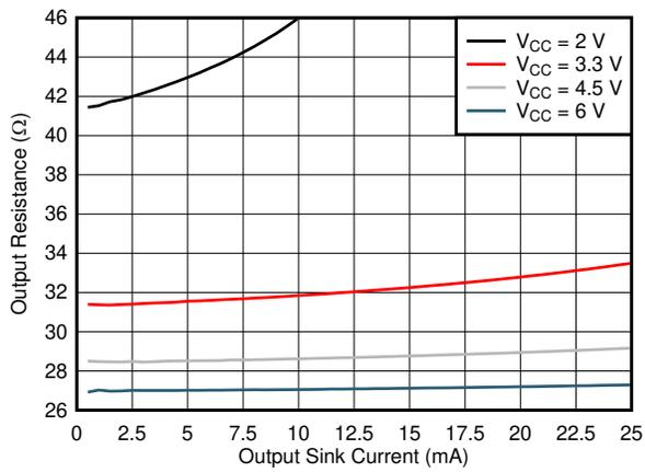
Figure 6-1. Output Driver Resistance in LOW State
