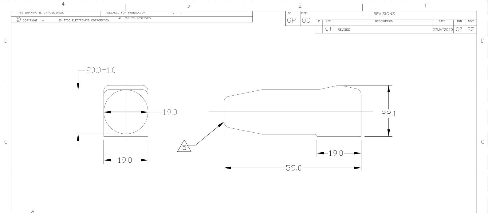
CABLE ENTRY OF BOOT IS MOULDED SOLID AND CROPPED TO SUIT CABLE USED BY CUSTOMER.
