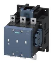
vacuum contactor, AC-3 225 A, 110 kW / 400 V AC (50-60 Hz) / DC operation 21-27.3 V AC/DC auxiliary contacts 2 NO + 2 NC 3-pole, frame size S10 busbar connections drive: electronic with PLC interface 24 V DC
