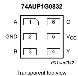
Fig. 4. Pin configuration SOT1115 and SOT1202 (XSON6)
