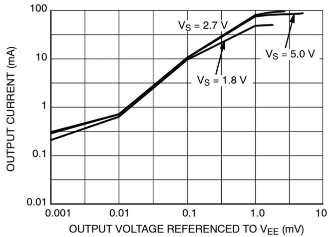
Figure 5. Sinking Current vs. Output Voltage
