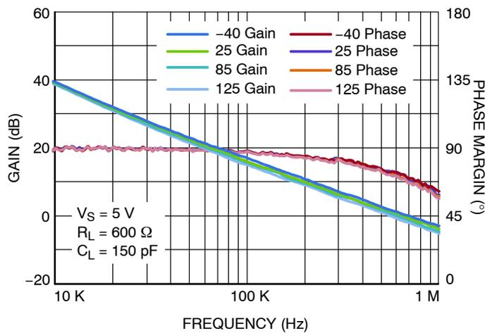
Figure 12. Gain and Phase vs. Temp
