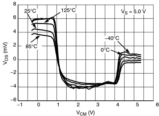
**Figure 28. Offset Voltage vs. Common Mode Range**
