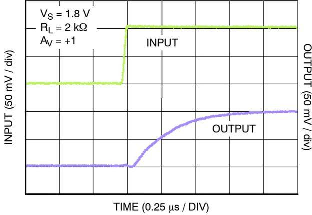
Figure 18. Small Signal Transient Response
