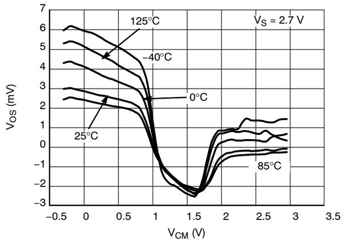
**Figure 27. Offset Voltage vs. Common Mode Range**
