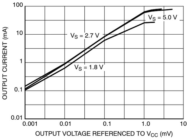
Figure 4. Sourcing Current vs. Output Voltage
