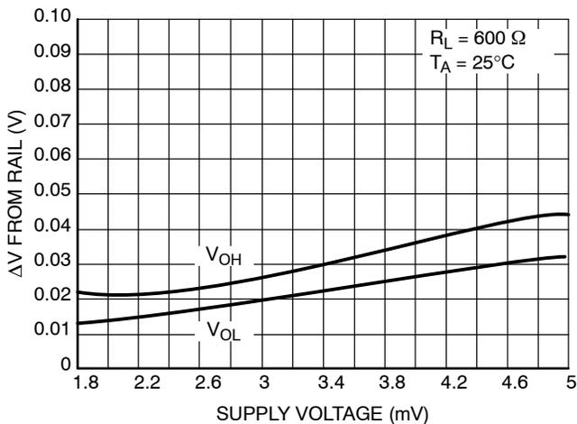
Figure 6. Output Voltage Swing vs. Supply Voltage
