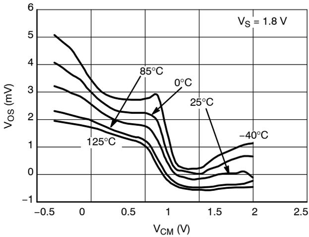
**Figure 26. Offset Voltage vs. Common Mode Range  $V_{DD}$**
