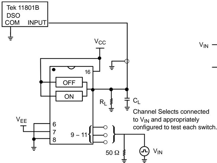
Figure 11. Break-Before-Make, Test Set-Up
