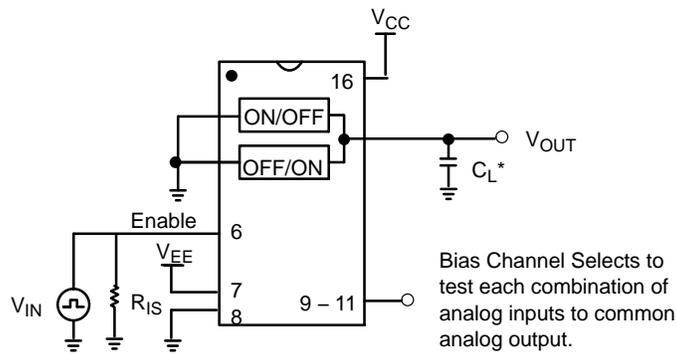
\*Includes all probe and jig capacitance.
