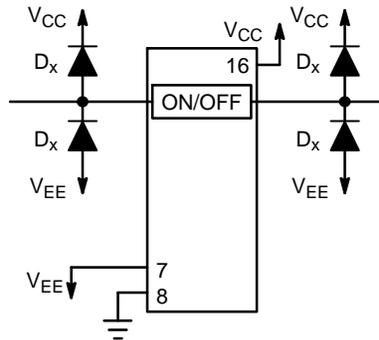
Figure 21. External Germanium or Schottky Clipping Diodes
