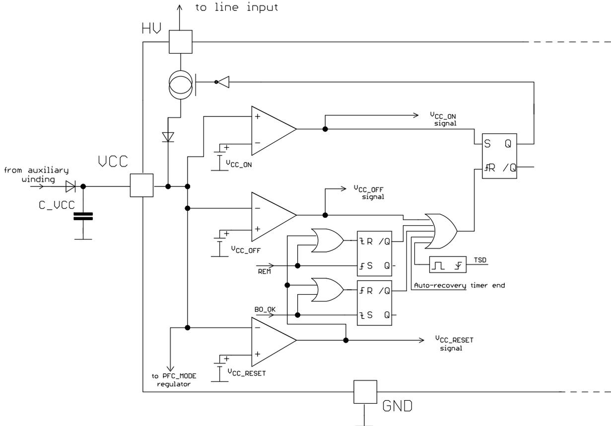
**Figure 4. Internal Connection of the VCC Management Block**
